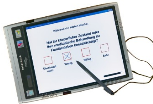
Figure 1: Example of an electronic questionnaire (EORTC QLQ-C30) using AnyQuest for Windows on a Tablet-PC. This computer measures about 33 cm x 22 cm x 2 cm (a little larger than a sheet of A4 paper) and can be linked to a practice- or hospital-IT-system via WLAN. The same software, however, also works on any older PC from 386/Windows 3.x/Linux etc., with or without a Touch-Screen.
